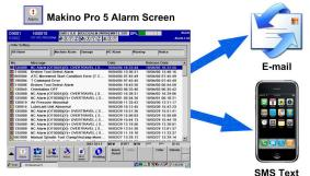
Remote Alarm Notification, allows <u>real-time monitoring of alarms and warnings</u>. It sends the information found on the Makino Pro 5<sup>®</sup> alarm screen to <u>email and</u> text messages as the alarms and warnings occur.
