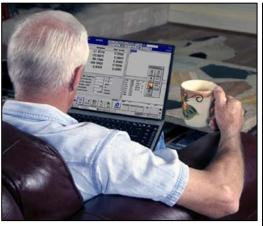
With Remote Machining you can view and control your Makino Pro 5 Mill from any internet connected PC in real-time. What you see and do on your PC while connected remotely is seen and done locally on the Mill itself. What an operator sees in the shop, you see remotely.
